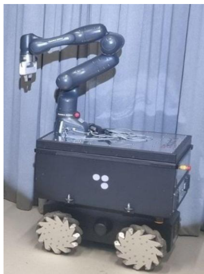
Mobile cobot (Franka Research III on Robotnik omniwheel base)
