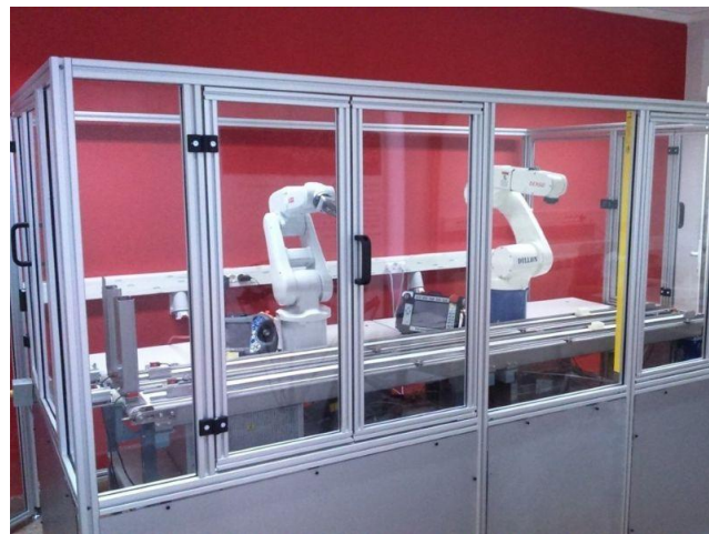
Cooperative industrial robot cell (by ABB, Denso and Siemens)
